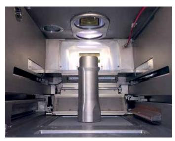
Fig. 4: Reactor built in the SLM\*280 selective laser melting machine
